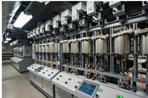
One-sample machines for creep tests manufactured by Ł-IMŻ
