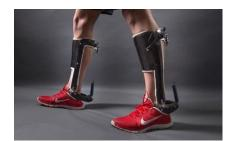
Walking with a passive-elastic ankle exoskeleton. An unpowered clutch engages a spring in parallel with the Achilles tendon when the foot is on the ground, offloading the calf muscles and making walking easier.
